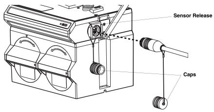
Figure 2-19 Connecting the AV Sensor
